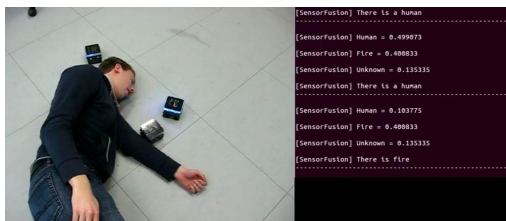
Figure 2: Application scenario. On the left side there is a victim which gets classified by the BeBots around it. On the right side there is the output of the sensor fusion.
