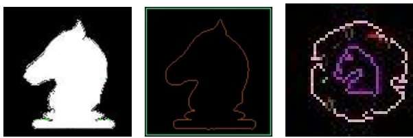
(a) Sample image of the chess piece to be matched (b) Contour of the image to be matched (c) Contour of the image from the video matched
