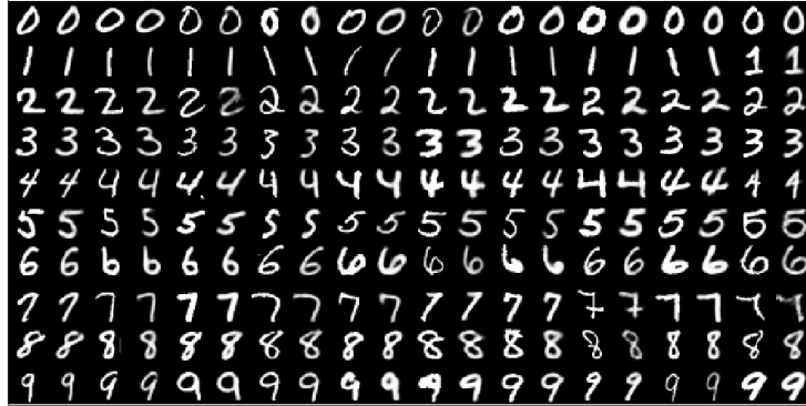
Figure 6: Reconstructed digits from the MNIST test dataset. From left to right: the digits are pairs of (original image, reconstructed image). For each digit we visualize 10 randomly chosen digits.
