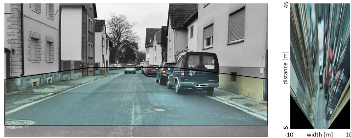
Fig. 2. Example image of BMAG camera. The colored area in the perspective view (left) denotes pixels inside the metric Bird's-Eye-View corridor (right).
