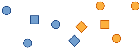
Figure 1: An illustration of prototype selection according to problem 1. Class labels are indicated by color. The optimal solution requires prototypes close to the classification boundaries (diamonds). The most representative prototypes would be the medoids (rectangles).
