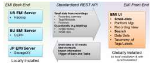
Figure 7: Overall EMI architecture
