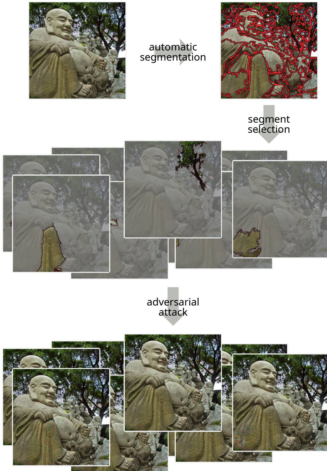
Figure 2: Overview of our process of generating multiple adversarial examples via localized adversarial attacks from a single input image. First, the image is automatically segmented. Then, the largest segments are chosen and individually used to constrain an adversarial attack.
