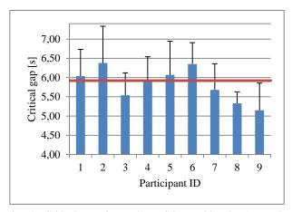
Fig. 4: Critical gap for each participant (blue bars), standard deviation of critical gap (black lines) and critical gap using data of all participants for estimation (red line).
