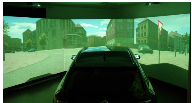
Figure 1: Static driving simulator at the Würzburg Institute for Traffic Sciences (WIVW), used for the user study.
