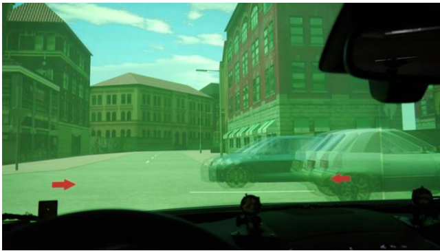
Figure 2: Simulated HUD display in the driving simulator with the coloured arrows visualizing traffic information from the left and right direction at an urban intersection
