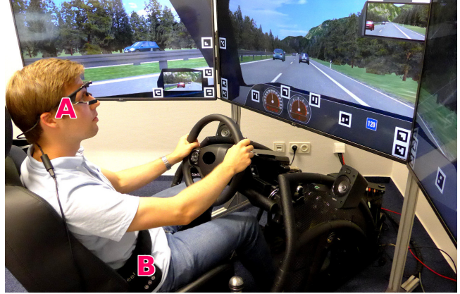
(a) Setup showing the driving simulator, eye-tracker (A), vibrotactile belt as LLI (B), and the driving scene from Figure 2 (T1).
