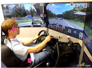
Figure 2: Experimental scenario showing the driving simulator, eye-tracker (A), vibrotactile belt (B), and the driving scene from figure 1.
