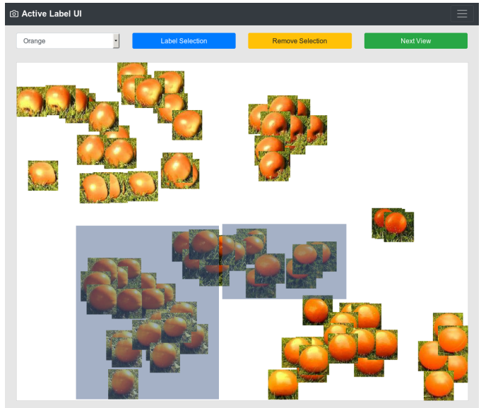
Fig. 3. Querying user interface showing a view queried by A2VQ. The user can label samples by selecting their thumbnails by dragging rectangles in the visualization. The class name can be entered in an input formula. There are certain possible strategies for labeling, like label everything, label only the biggest clusters or label only outliers. With a click on the button Query next view the classifier is retrained with the new labeled samples and a new view is queried with A2VQ.
