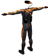
Fig. 1: The XSENS body suit with seventeen IMU sensors. The sternum IMU is occluded due to the image perspective. We used the wireless version. Source: https://www.xsens.com/ .
