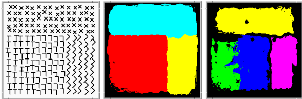
Figure 7. Grouping of textures consisting of L’s T’s and x’s: Similar to the untrained human observer the CLM only distinguishes between three different regions in (b). In (c) we decreased the parameter R_{sim} in (7), such the model “looks closer at texture differences” and perceptually organizes the image in four distinct groups.
