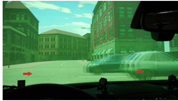
Fig. 4. Simulated HUD display in the driving simulator with the colored arrows visualizing traffic information from the left and right direction at an urban intersection.
