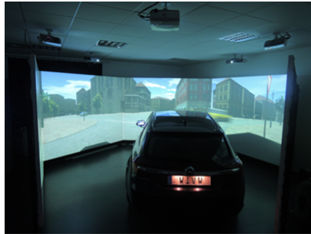
Fig. 1. Outside view of the static driving simulator of WIVW used for the study.
