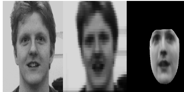
Fig. 12. Synthesising a high-res face from a low-res sequence. Left hand image: an original frame from sequence. Centre image: frame from deliberately blurred sequence. Right hand image: final reconstruction from low-res sequence
