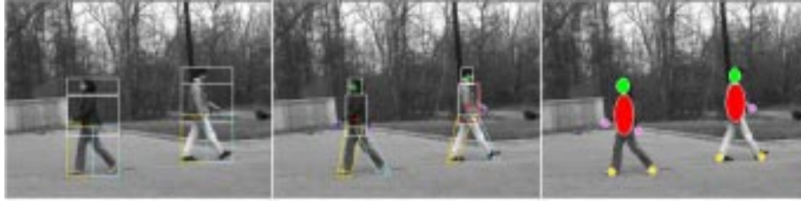
Fig. 11. An example of Cardboard Model to show How Head, Torso, Legs Hands and Feet are Located. Initial Bounding boxes are located on foreground regions (a); Cardboard model analysis locates the body part (b); illustration of body part location by ellipsis (c)
