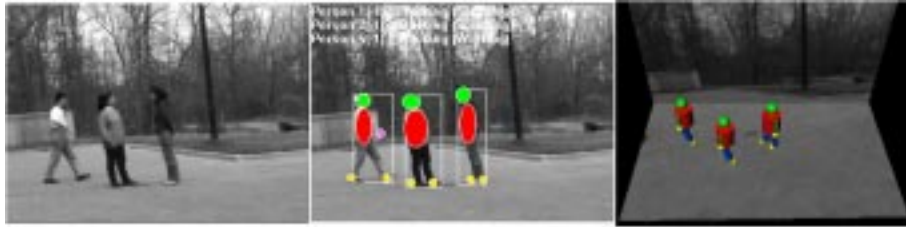
Fig. 1. Examples of detection result: intensity image (left), detected people and their body parts from the intensity only (middle) and their placement in the 2\frac{1}{2}D scene by W^4S (right)
