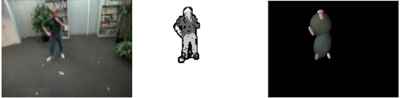
Figure 1: (left) video input (n.b. color image shown here in greyscale), (center) segmentation, (right) a 2-D representation of the blob statistics
