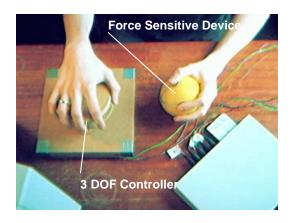
Fig. 1. A dual-hand interface developed for multiparametric control of speech
