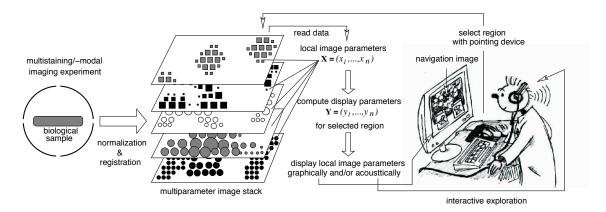
Fig. 1. The set up of interactive exploration of multiparameter images with visualization and sonification methods
