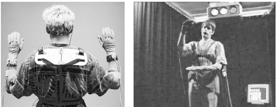
Fig. 2. Gesture and speech recording devices (left): Data gloves, motion trackers, and microphone headset. Example from the corpus (right): Showing the vertical extent of an object
