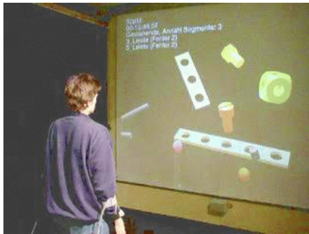
Fig. 5. The prototype system: Selecting reference objects by gestural shape description
