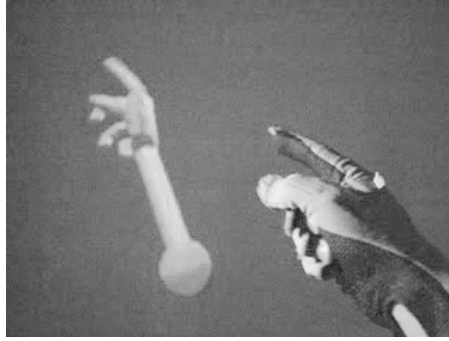
Fig. 6. Visualization of hand model (left) and real hand with CyberGlove (right)
