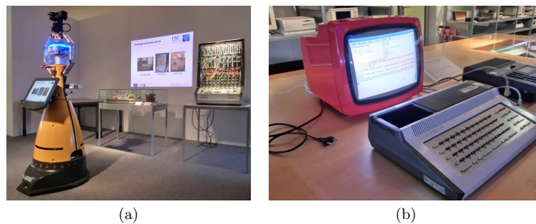
Fig. 1. Two possible scenarios of augmented reality with our robot: (a) Robot projecting to a plain wall, (b) Robot projecting onto a CRT display, 'reviving' the old hardware.
