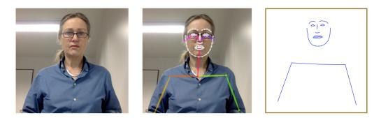
Figure 1: Extracting movement features with Open Pose based on body, hand, and face recognition.
