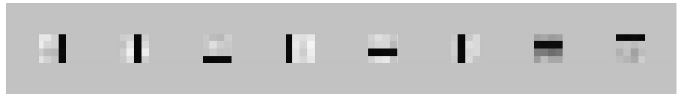
Fig. 2. Solution of the standard NMF algorithm for 8 basis vectors. The basis vectors comprise all 4 horizontal and all 4 vertical lines. The transformation properties of the input are encoded implicitly in the basis vectors; they are translated versions of each other. To the contrary, the overlapping NMF algorithm would consider the translations explicitly, and only 2 basis vectors would be needed: One horizontal and one vertical. The input is then reconstructed by shifting these basis vectors to all of their 4 possible positions.
