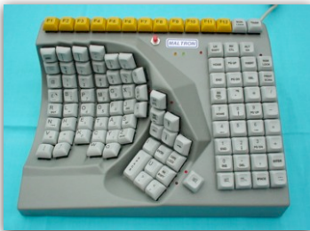
Maltron left-handed keyboard for one handed use
