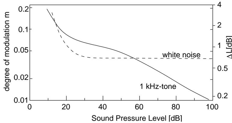
Figure 4.5: Resolution of loudness perception as a function of the sound level (modified from [ZF99]).
