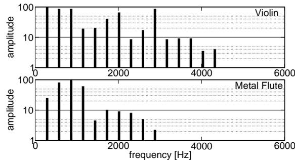
Figure 8.20: Timbre of two musical instruments, characterized by their timbre vectors. The plot shows the amplitudes of the partial tones, which are also called harmonics. Data from [BS74].
