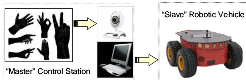
**Figure 2.** Gestural teleoperation of a mobile robotic vehicle: “Desktop” scenario.
