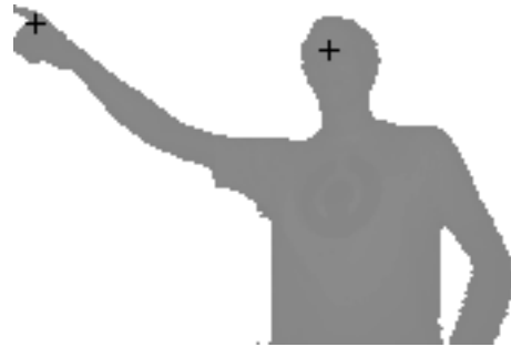
Fig. 1. Segmented image of the user with the detected locations of the head and hand marked by crosses. The time-of-flight camera measures the three-dimensional positions of these points, which are then used to compute the pointing direction.
