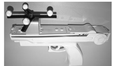
Figure 2: Nintendo Wii Remote extended by a pistol grip
