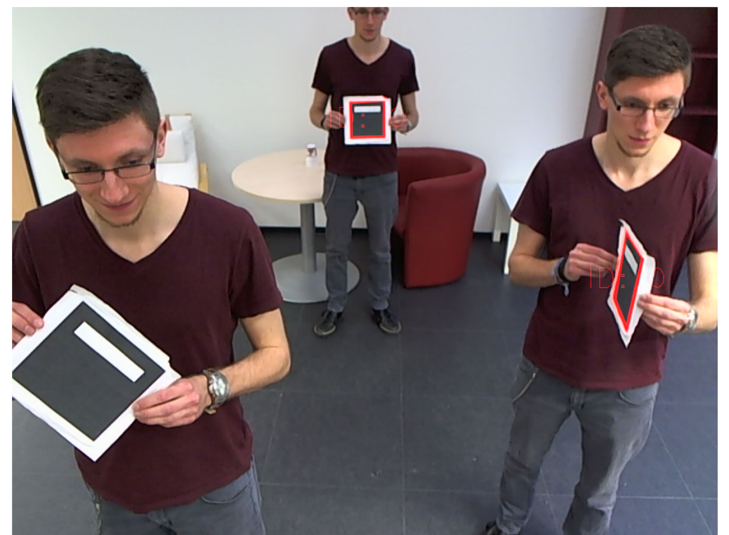
Figure 2: Various border cases of our marker tracking approach. Left: An arbitrary small part of the marker leaves the camera's viewport. Middle: The farthest point, where the marker can still be seen by our tracking application. Right: Even if the marker is orientated almost parallel to the camera's viewing axis, it can still be tracked.
