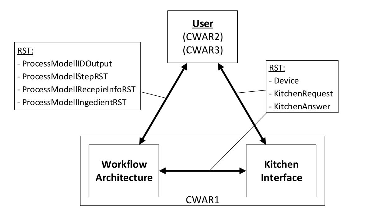
Figure 2: Communication between different project parts with RSB.
