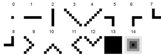
Figure 6. Connection weight patterns for local feature detection. Black denotes a connection weight of 1.0, white a connection weight of  $-1.0$ , and the gray scales denote connection weights between  $0.0$  and  $1.0$ .
