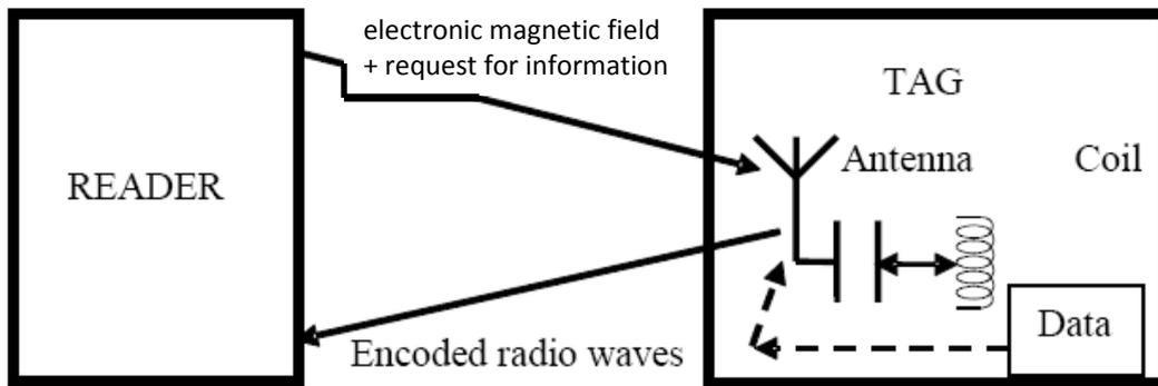
Figure 1 Passive RFID
