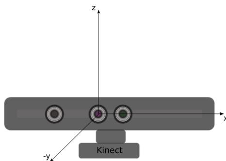
Figure 1: The world coordinate system as defined by the Kinect camera and the tracking software OpenNI & NiTE.
