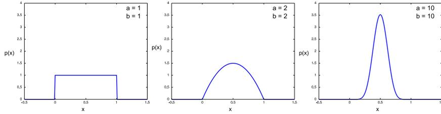
Fig. 2: Beta distribution used to study the accuracy and robustness of the classical and the ensemble GMM. The beta distribution takes the form of a uniform distribution in case the two parameters are set to  $a = b = 1$  (left plot). Parameters set to  $a = b = 2$  result in a concave shape with a rough change on the boundary of its support (middle plot). A shape close to a Gaussian distribution is obtained setting the parameters to  $a = b = 10$  (right plot).
