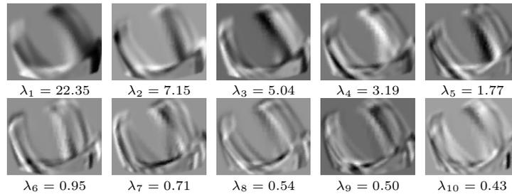
**Fig. 2.** The 10 principal eigen-images and the corresponding eigenvalues. Note that the values were scaled to be in the range  $[0; 1]$ .
