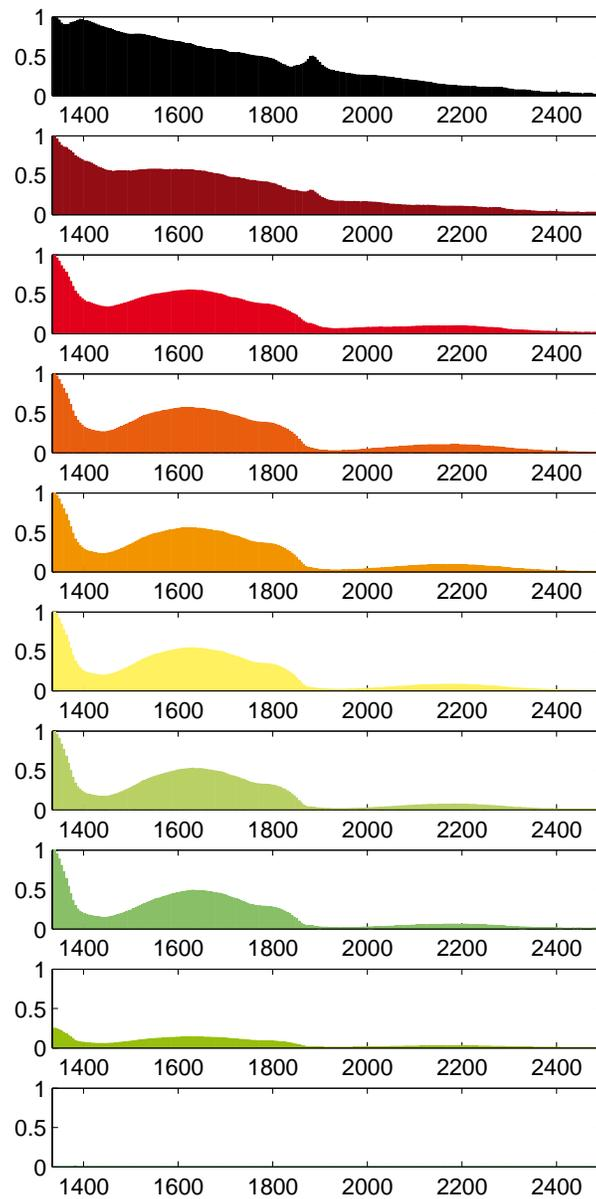
**Fig. 4.** Result of the Neural Gas training: normalized weight vectors of 10 neural prototypes, sorted according to their similarity (top to bottom), representing the centers of the 10 clusters. These prototypes also represent characteristic hyperspectral fingerprints formed from the data set during network training (abscissa shows the wavelength in nm). Figure borrowed from [9].
