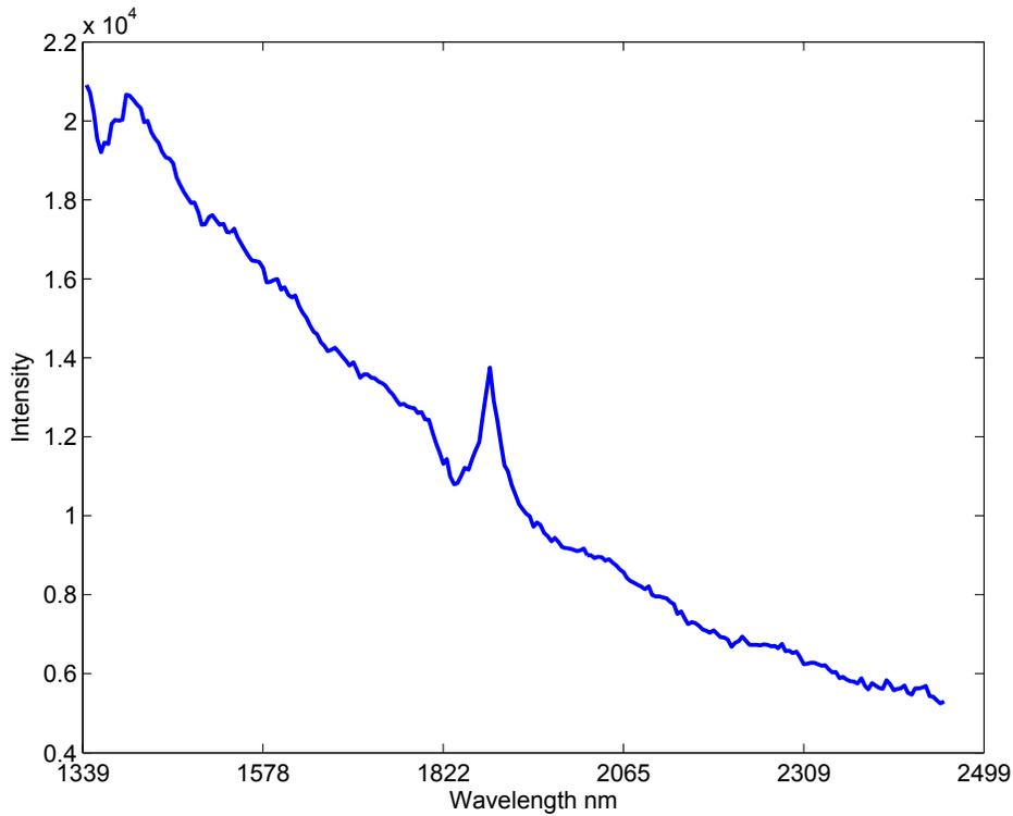
**Fig. 1.** Spectral intensity reflected by the used calibration normal (100%-reflection type, polytetrafluoroethylene (PTFE) pad). The typical physical effect of decreased reflected energy with increasing wavelengths can be clearly observed. The actual gradient of this curve depends on the specific characteristics of the measurement equipment, such as sensor, lens, and illumination source. This curve is used to normalize all acquired images of the scenery.
