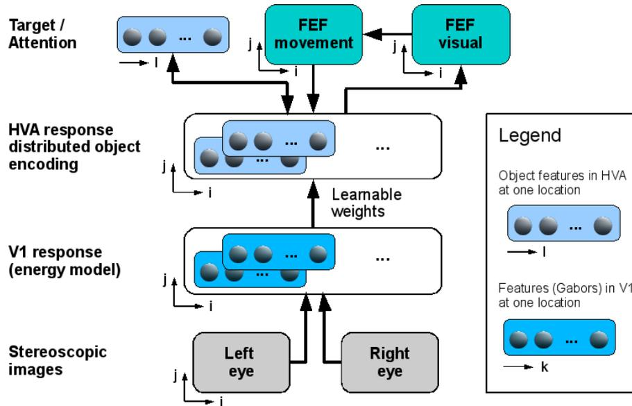
**Fig. 2.** Neuronal network of the stereoscopic object recognition model. The  $i$  and  $j$  indices correspondent to the spatial  $x$  and  $y$  axis of the images. The index  $k$  refers to different Gabor responses and  $l$  to different learned features in HVA.
