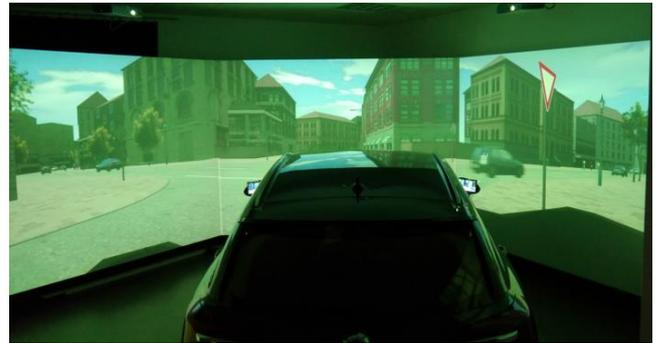
Fig. 1: Static driving simulator at the Würzburg Institute for Traffic Sciences (WIVW) used for the user-study.
