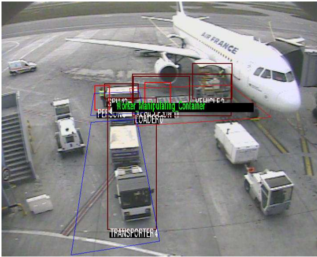
Figure 5. (Left) Two dynamic zones (in blue) linked with the Loader and the Transporter vehicles involved in the detected event “Worker.Manipulating.Container” (event 26). (Right) The Unloading operation involves 8 physical objects and 3 composite components with 2 constraints on the vehicle subtypes, 4 constraints on the zones of interest and 2 temporal constraints.
