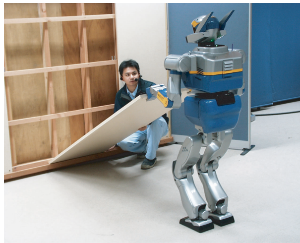
Fig. 13. HRP-2 assembles a cottage with a human.
