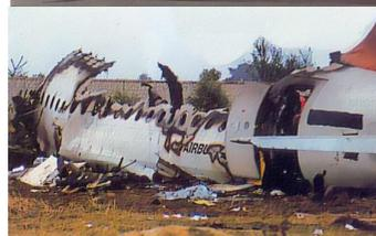
"The pilot put the plane into OPEN DESCENT mode without realizing it. This change resulted in the aircraft's speed being controlled by pitch rather than thrust. The throttles went to idle. In that mode, the automation ignores any preprogrammed altitude constraints. To maintain the pilot-selected speed without power, the automation had to use an excessive rate of descent, which led to a crash short of runway."
