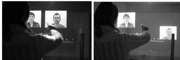
**Figure 3: Example interaction with the HoloPro™ prototype: the right ISD is sent to the back with a tap of a finger (perspectively correct for the user's view, however not for the camera taking the picture).**
