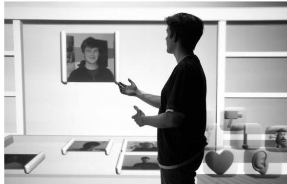
**Figure 1: The ISDs in the immersive Virtual Reality set-up. Interlocutors are represented by scroll-like panels floating in the air. The layout of the ISDs can be arranged by the user.**
